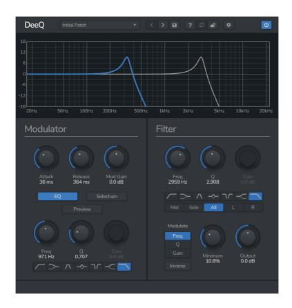
DeeQ is a single band mid/side dynamic EQ. With DeeQ you can not only set the band's frequency, Q, and gain, but you can also modulate them using the incoming audio or an external sidechain, and set the band to operate in mid/side or stereo mode.
